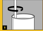
Thoroughly mix the Ready Roof liquid rubber using the paddle whisk provided on a low speed setting with your electric battery driver so as not to introduce air bubbles into the liquid. Ensure there are no separations and any settlements at the bottom of the tin are completely dispersed so that the liquid is uniform in appearance and colour.
