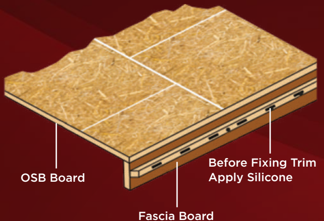
Diagram 5 - Water run off required Drip Fascia Trim
